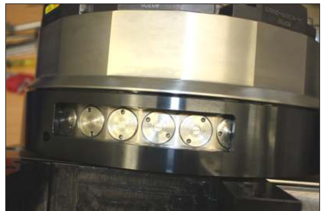
(2) Coupling nipples in the revolver fixture (total 36 coupling nipples)
